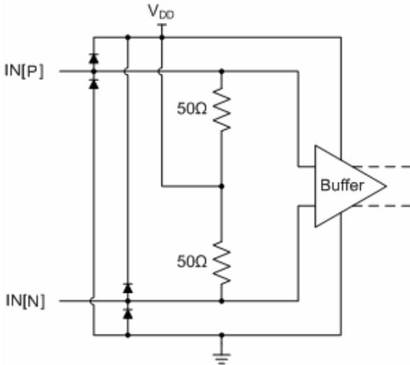
FIGURE 6. CML INPUT EQUIVALENT CIRCUIT FOR THE QLx111GRx
