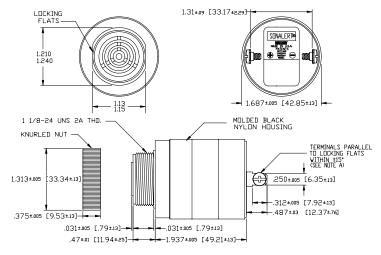
NDTE A: TERMINALS-032 BRASS TIN PLATED, TAPPED FOR #6-32 SCREW. TWO #6-32 NICKEL PLATED BRASS SCREWS INCLUBED. WILL ACCEPT 1/4' QUICK CONNECT.
