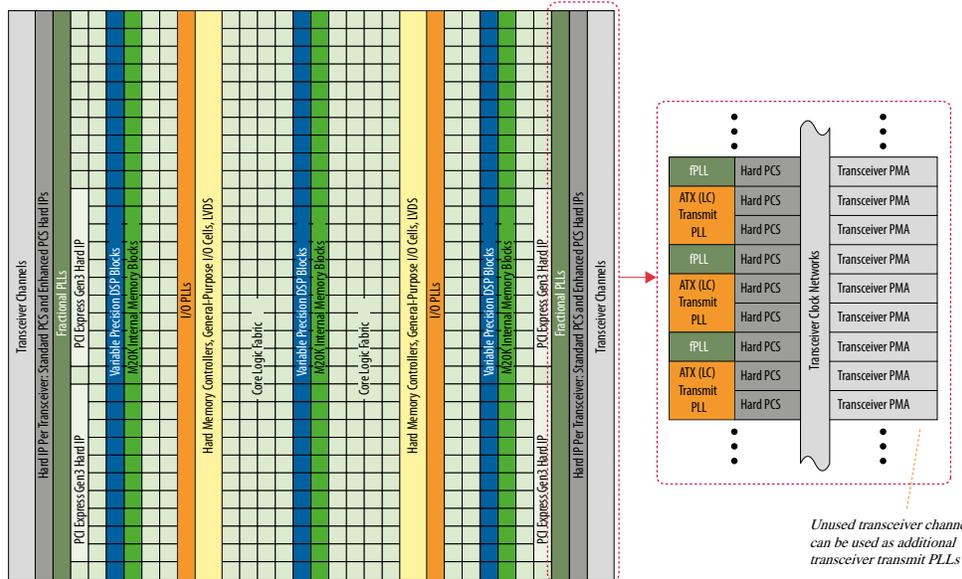
Figure 8. Device Chip Overview for Arria 10 SX Devices
