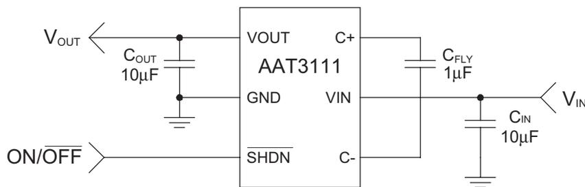
**Figure 6: Typical Charge Pump Boost Converter Circuit.**
