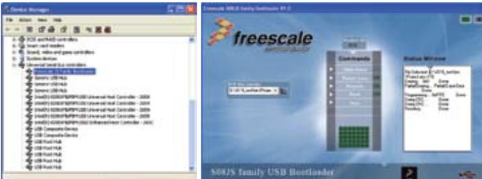
5. Open the family bootloader V1.0 GUI using the path “Start>Programs>Freescale>JS Family Bootloader.” The USB bootloader GUI is shown above.
