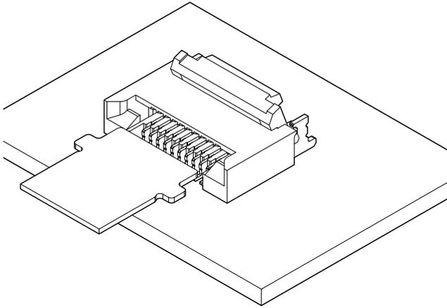
**This is 2.0mm height connector with the double-sided contact for FPC. As FPC with protrusions is used for this FHH connector, prevention of incomplete insertion and mis-insertion are realized and connection reliability is improved.**
