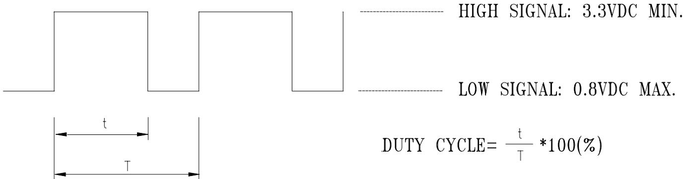
THE FREQUENCY FOR CONTROL SIGNAL OF THE FAN SHALL BE ABLE TO ACCEPT A 10KHZ.
