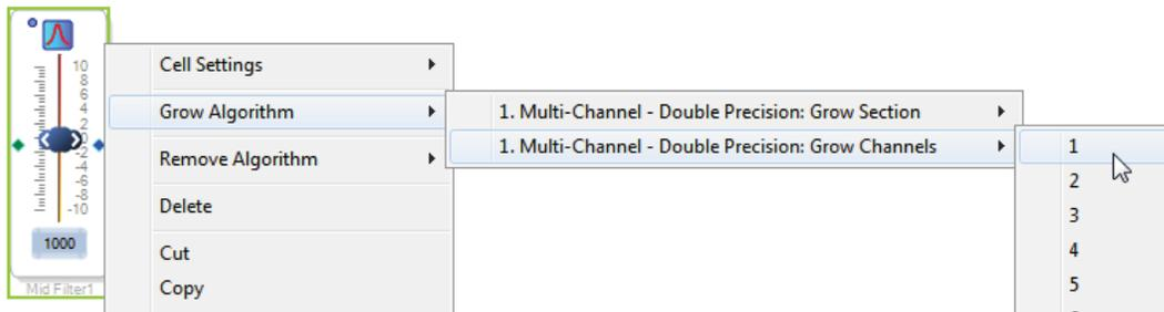
Figure 52. Adding a Channel to the Filter
