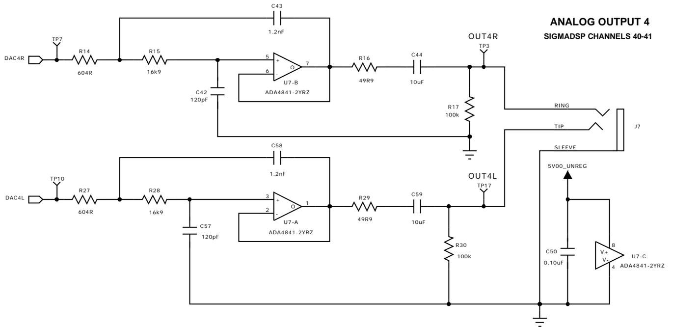
Figure 84. Analog Output Channel 40 and Channel 41
