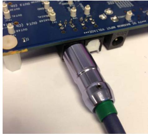
Figure 34. Photograph of the Optical S/PDIF Input Connection
