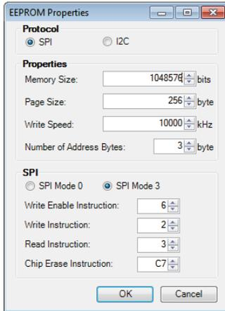
Figure 65. EEPROM Properties Window and Required Settings
