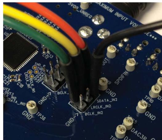
Figure 57. Connecting External I<sup>2</sup>S Signals to Serial Input Port 2
