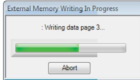
Figure 66. External Memory Write Operation Status Window
