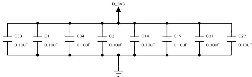
Figure 85. Plane Decoupling Capacitors
