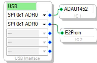
Figure 63. E2Prom Setup in Hardware Configuration Tab
