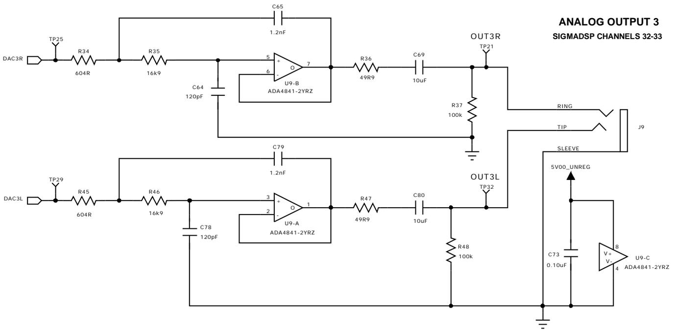
Figure 83. Analog Output Channel 32 and Channel 33
