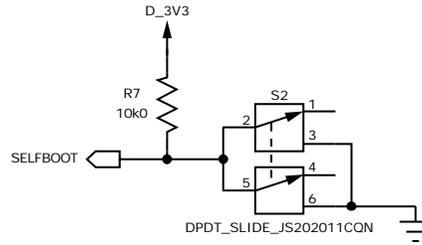
Figure 72. Self-Boot Circuit
