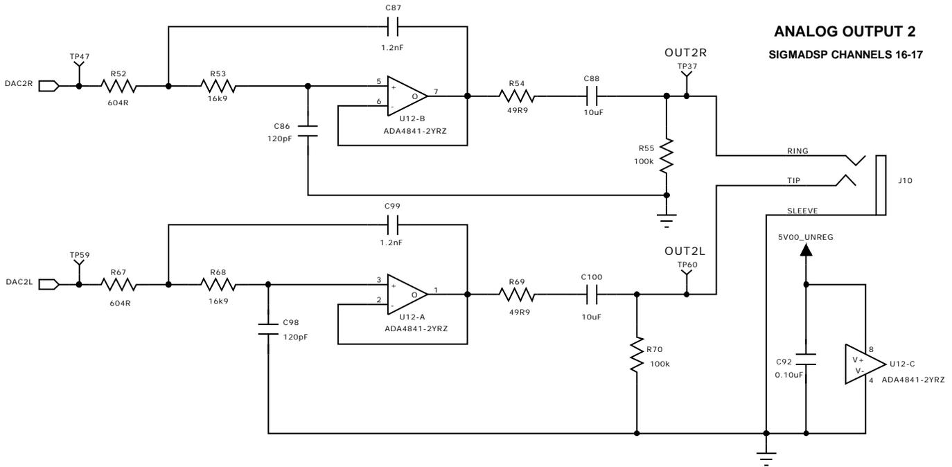
Figure 82. Analog Output Channel 16 and Channel 17
