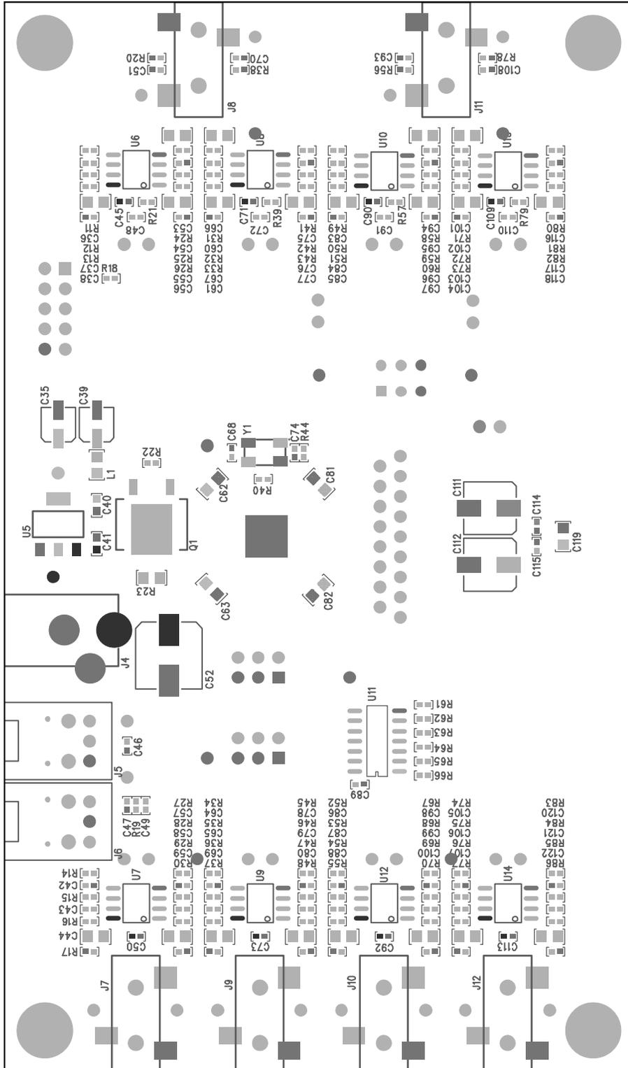
Figure 92. EVAL-ADAU1452MINIZ Layout, Bottom Assembly (Viewed from Below)
