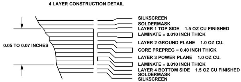
Figure 93. Cross Section of PCB Stack Up
