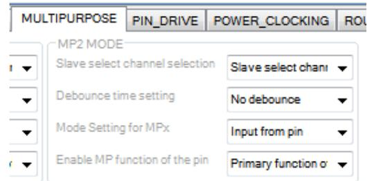
Figure 59. Multipurpose Pin Configuration in SigmaStudio
