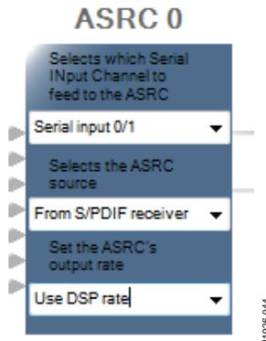
Figure 42. Configuring the ASRC 0 Routing Matrix Registers
