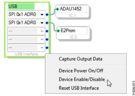
Figure 69. Toggling the Reset Signal in SigmaStudio
