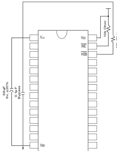
In system power mode, both V<sub>CC</sub> and V<sub>CAP</sub> are connected to the +5 V power supply without the 68 μF capacitor. In this mode, the AutoStore function of the STK12C68 operates on the stored system charge as power goes down. The user must, however, guarantee that V<sub>CC</sub> does not drop below 3.6 V during the 10 ms STORE cycle.
