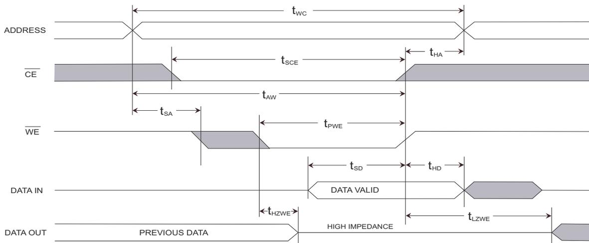
Figure 10. SRAM Write Cycle 2:  $\overline{CE}$  Controlled [11, 12]
