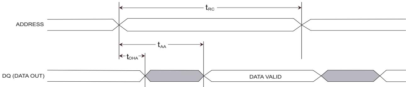
Figure 8. SRAM Read Cycle 2:  $\overline{CE}$  and  $\overline{OE}$  Controlled [7]
