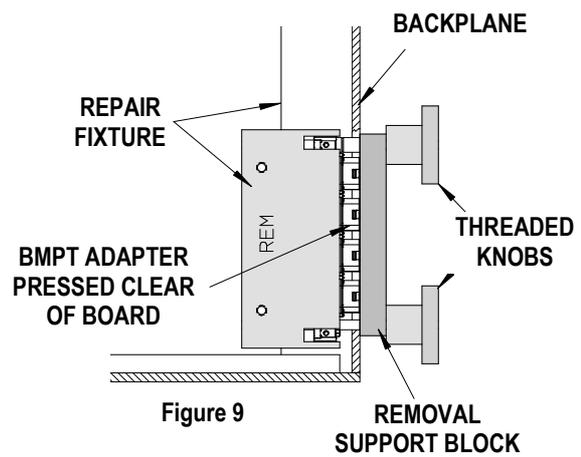
9. Turn both knobs until the damage adaptor is pressed out of the backplane. See Figure 9.
