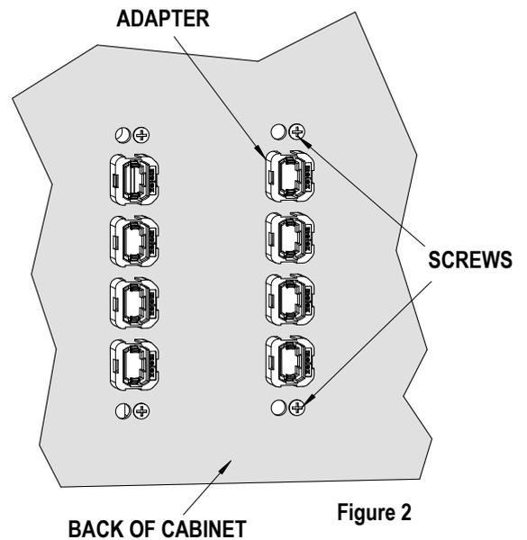
2. With a screwdriver remove the two (2) small Phillips head screws holding the assembly in place. See Figure 2.
