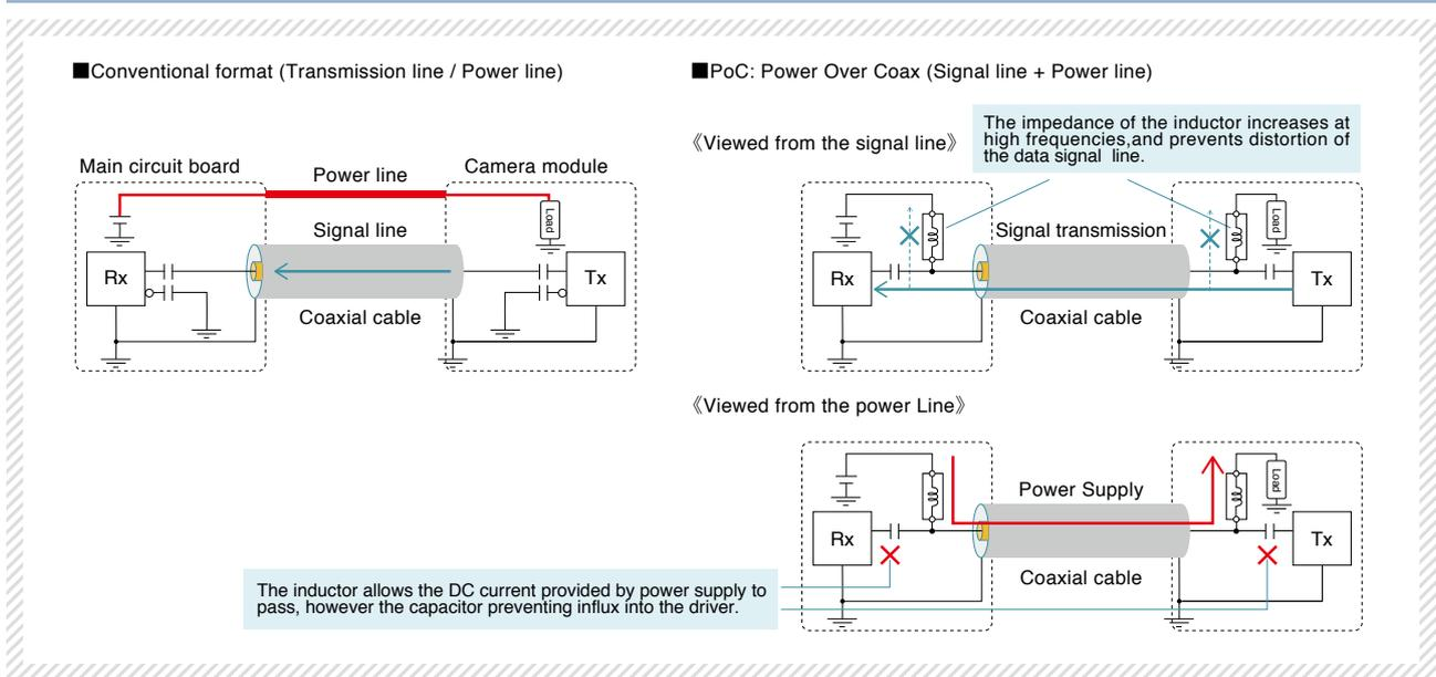
**Characteristics and composition required of an inductor for use with in-vehicle PoC**
