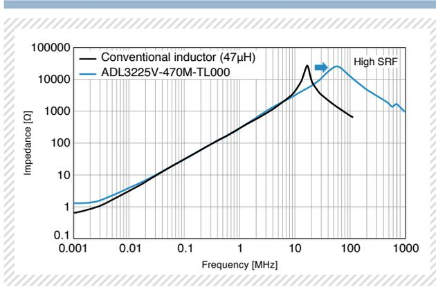
**Realizing Broadband Impedance Characteristics and Good DC Superimposition Characteristics**
