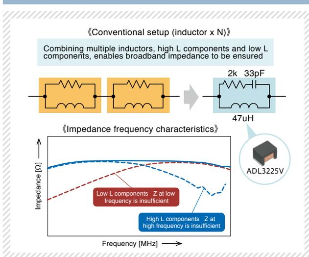
The product that provides the solution to these required characteristics is the ADL3225V type that raises the self-resonant frequency, together with achieving the DC superimposition characteristics, by adopting the original coil design and construction different to that of conventional power inductor.
