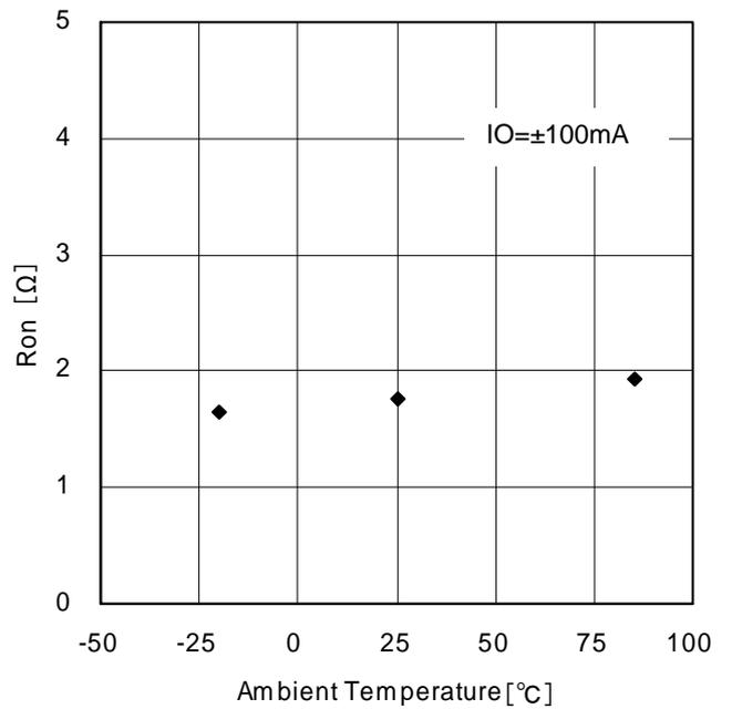
Figure 8. Output ON-Resistance Temperature Dependency (Voltage driver block)
