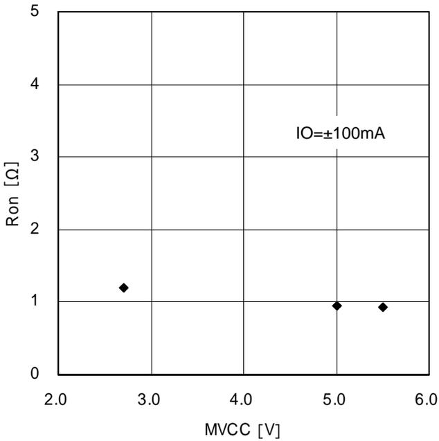
Figure 9. Output ON-Resistance
