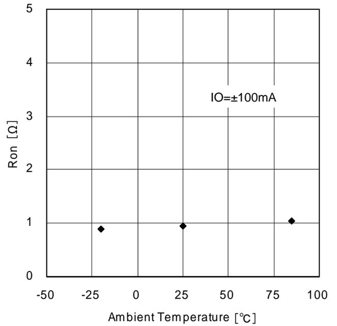
Figure 10. Output ON-Resistance
