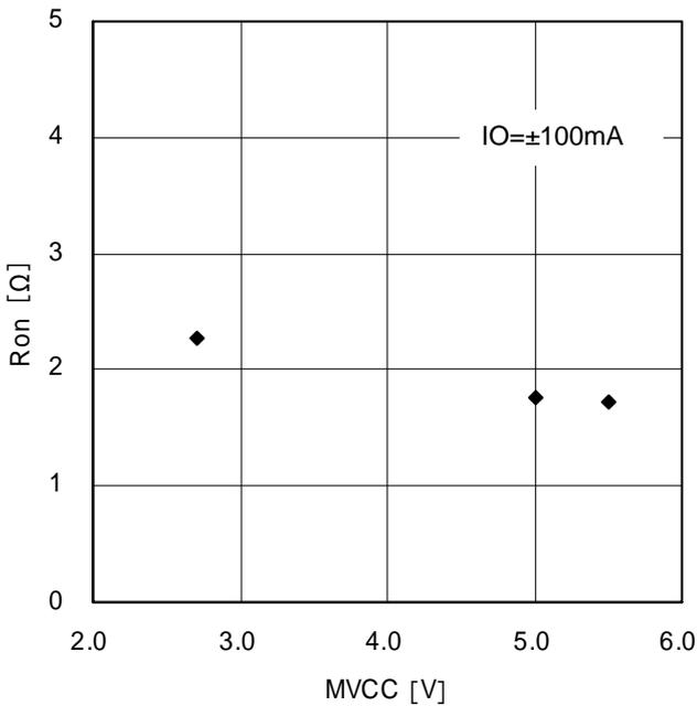
Figure 7. Output ON-Resistance MVCC Dependency (Voltage driver block)
