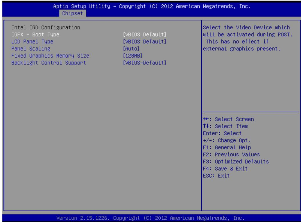
Figure 3.16 Intel IGD Configuration
