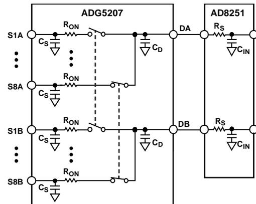
Figure 4. Settling Time Model of the ADG5207
