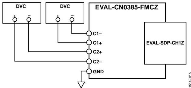
Figure 15. Settling Time Evaluation Setup Using DC Calibrators
