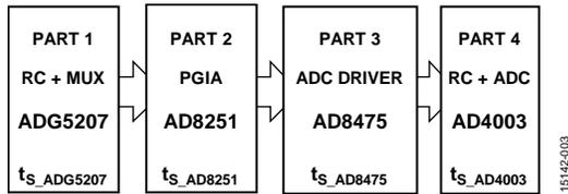
Figure 3. Settling Time Model of CN-0385 Circuit
