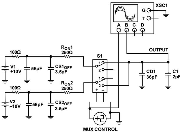
Figure 5. Multisim Settling Time Model of the ADG5207
