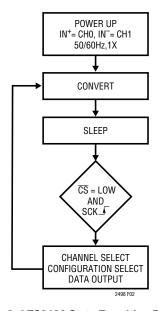
Figure 2. LTC2498 State Transition Diagram
