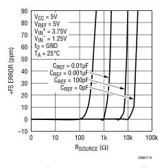
Figure 14. +FS Error vs R<sub>SOURCE</sub> at V<sub>REF</sub> (Small C<sub>REF</sub>)
