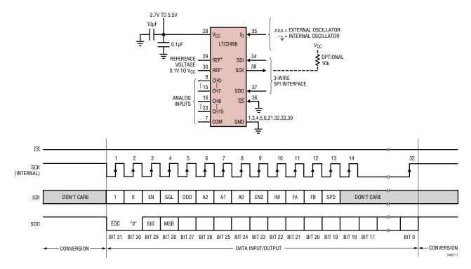
Figure 11. Internal Serial Clock, Continuous Operation
