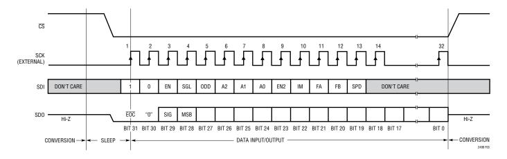
Figure 3. Channel Selection, Configuration Selection and Data Output Timing
