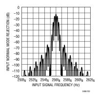
Figure 22. Input Normal Mode Rejection at f<sub>S</sub> = 256 • f<sub>N</sub>
