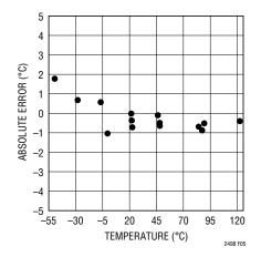
Figure 5. Absolute Temperature Error
