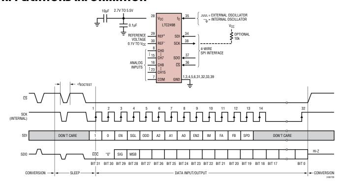
Figure 9. Internal Serial Clock, Single Cycle Operation
