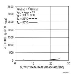
Figure 32. +FS Error vs Output Data Rate and Temperature
