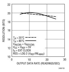
Figure 35. Resolution (INL<sub>MAX</sub> ≤ 1LSB) vs Output Data Rate and Temperature
