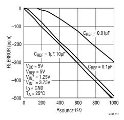
Figure 17. -FS Error vs R<sub>SOURCE</sub> at V<sub>REF</sub> (Large C<sub>REF</sub>)
