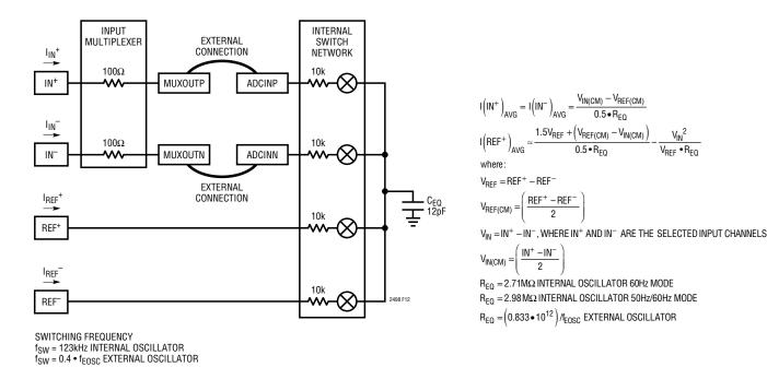
Figure 12. LTC2498 Equivalent Analog Input Circuit
