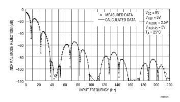
Figure 25. Input Normal Mode Rejection vs Input Frequency with Input Perturbation of 100% (50Hz/60Hz Notch)
