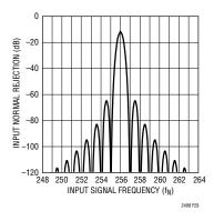
Figure 29. Input Normal Mode Rejection 2x Speed Mode
