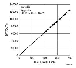
Figure 4. Internal PTAT Digital Output vs Temperature
