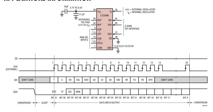
Figure 8. External Serial Clock, 3-Wire Operation ( $\overline{CS} = 0$ )
