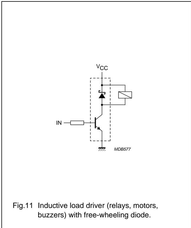
NPN transistor/Schottky-diode module
