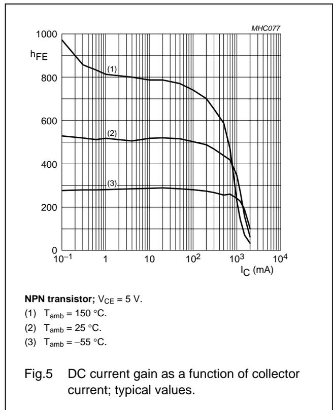
NPN transistor/Schottky-diode module
