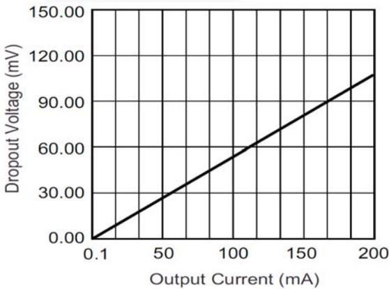
Figure 19. Dropout Voltage
