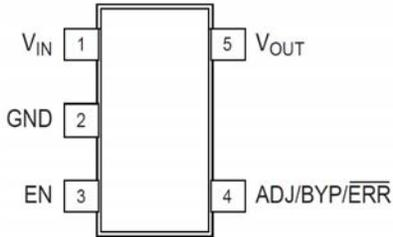
Figure 2. Pin Configuration
