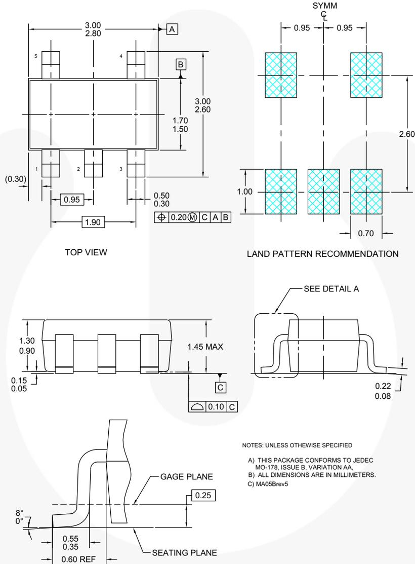
Figure 26. 5-LEAD, SOT-23, JEDEC MO-178, 1.6 mm
