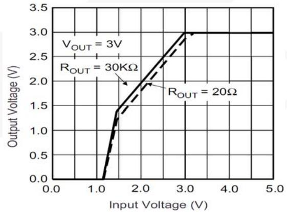
Figure 20. Dropout Characteristics
