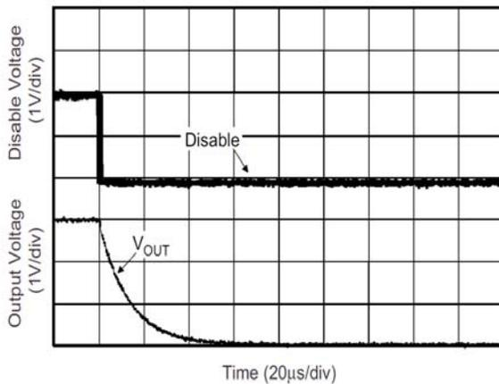
Figure 25. Shutdown Delay
