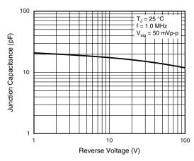
Figure 5. Typical Junction Capacitance
