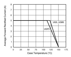
Figure 1. Forward Current Derating Curve
