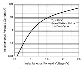
Figure 4. Typical Instantaneous Forward Charateristics
