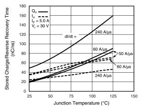
Figure 6. Reverse Switching Characteristics
