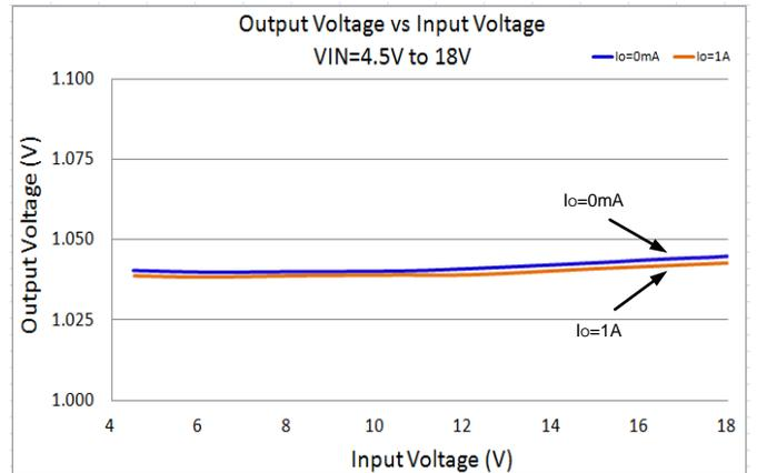
**Typical Performance Characteristics** (continued) (@T<sub>A</sub> = +25°C, V<sub>IN</sub> = 12V, V<sub>OUT</sub> = 1.05V, unless otherwise specified.)
