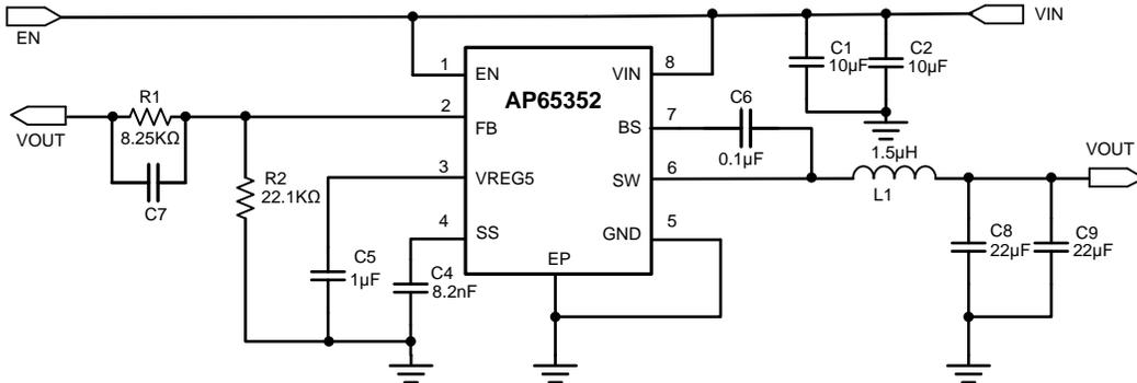
Figure 3 Typical Application of AP65352 evaluation board
