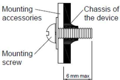
■ Only use M3 screw  $\leq$  6 mm through the base mounting holes. This is to keep a safe distance between the screw and internal components.
