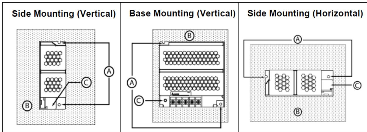
Fig. 2 Mounting Orientation
