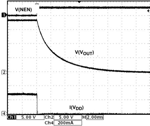
FIGURE 8. SHUTDOWN ( $V_{DD} = 3.6V$ ,  $R_L = 360\Omega$ )
