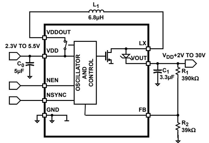
NOTE:  $V_{OUT} = (390k + 39k)/39k * 1.15V = 12.65V$
