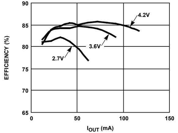
FIGURE 3. EFFICIENCY vs  $I_{OUT}$  ( $V_{OUT} = 18.3V$ )
