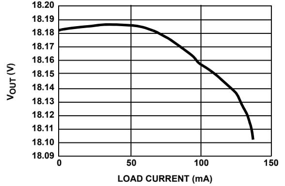
FIGURE 9. LOAD REGULATION ( $V_{IN} = 3.6V$ )
