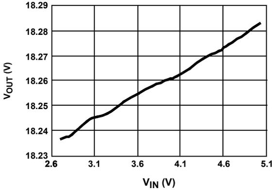
FIGURE 10. LINE REGULATION ( $I_{OUT} = 30mA$ )
