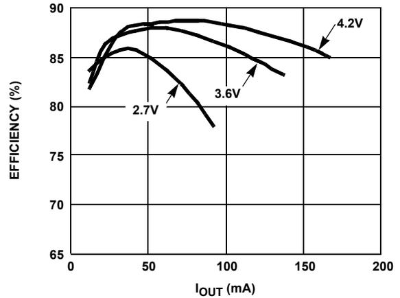
FIGURE 5. EFFICIENCY vs  $I_{OUT}$  ( $V_{OUT} = 12.7V$ )
