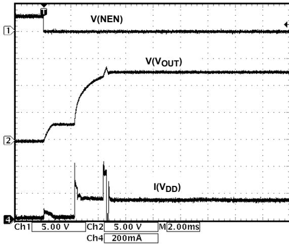
FIGURE 6. START-UP TO 12V ( $V_{DD} = 3.6V$ ,  $R_L = 360\Omega$ )
