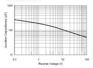
Figure 5. Typical Junction Capacitance
