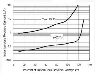
Figure 3. Typical Reverse Characteristics per Leg
