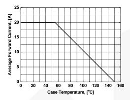
Figure 1. Maximum Derating Curve for Output Current
