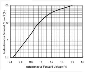
Figure 4. Typical Forward Characteristics per Leg
