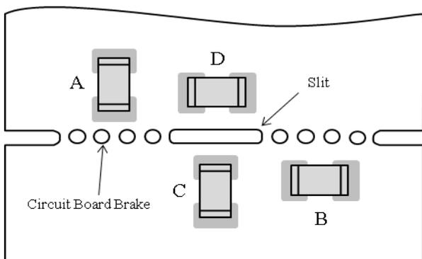
Stress strength according to the mounting position:
