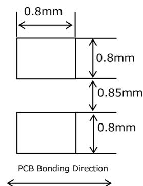
※The product has adopted the electrode structure that it should solder with back electrode of the product.
