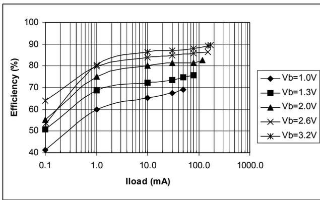
Figure 1. Efficiency Vs Output Current (Vout = 3.3V) Rlim=2.5K
