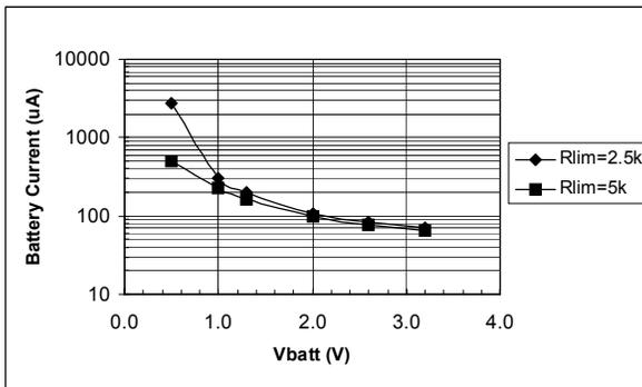
Figure 5. No-Load Battery Current Vs Vbatt (Vout = 3.3V)
