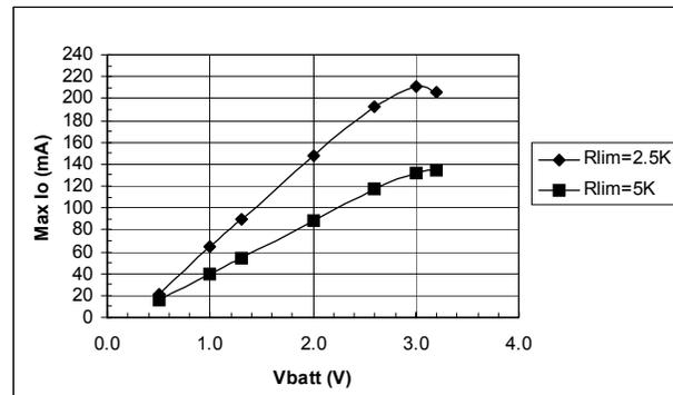
Figure 6. Maximum Load Current Vs Vbatt (Vout = 3.3V)
