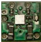
Figure 1. SSM2317 Evaluation Board Top View
