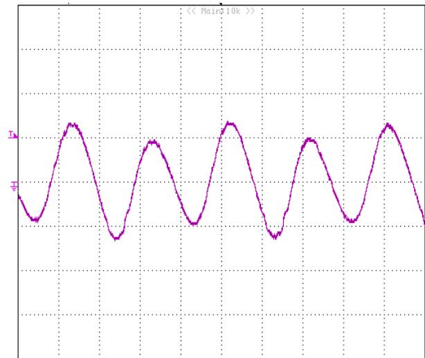
**Figure 11:** Input Terminal Ripple Current,  $i_c$ , at full rated output current and nominal input voltage with  $12\mu H$  source impedance and  $100\mu F$  electrolytic capacitor (500 mA/div, 2us/div).
