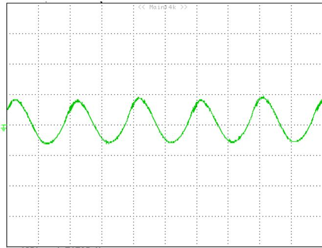
**Figure 14:** Output voltage ripple at nominal input voltage and rated load current ( $100\text{ mV/div}$ ,  $2\mu\text{s/div}$ )
