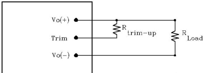
**Figure 17:** Circuit configuration for trim-up (increase output voltage)
