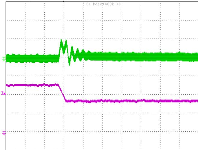
**Figure 8:** Output voltage response to step-change in load current (75%-50% of  $I_{o, \max}$ ;  $di/dt = 0.1A/\mu s$ ,  $V_{in}=54V$ ). Load cap:  $10\mu F$ , tantalum capacitor and  $1\mu F$  ceramic capacitor. Top Trace:  $V_{out}$  (200mV/div, 200us/div); Bottom Trace:  $I_o$  (10A/div, 200us/div). Scope measurement should be made using a BNC cable (length shorter than 20 inches). Position the load between 51 mm to 76 mm (2 inches to 3 inches) from the module.
