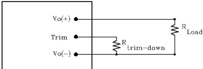
**Figure 16:** Circuit configuration for trim-down (decrease output voltage)
