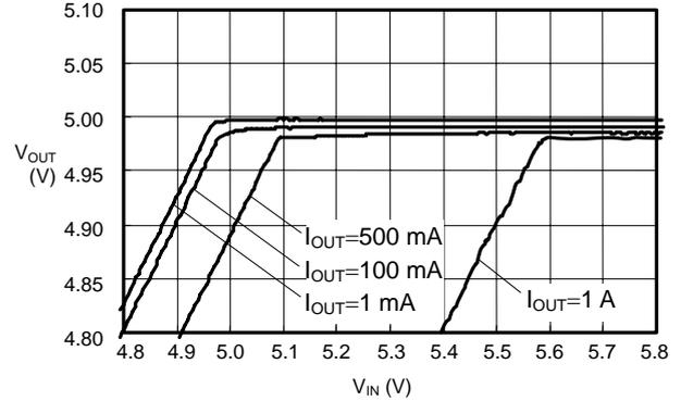
**2. Output Current ( $I_{OUT}$ ) - Output Voltage ( $V_{OUT}$ ) Characteristics**
