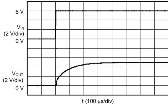
2. Input Transient Response Characteristics (Supply voltage variation  $V_{IN}=V_{OUT}+1\text{ V} \leftrightarrow V_{OUT}+2\text{ V}$ ,  $C_L=10\text{ }\mu\text{F}$ )
