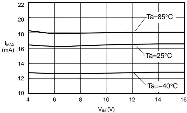
**6. Input Voltage ( $V_{IN}$ ) - Shutdown Pin Input Voltage ( $V_{SH}$ ,  $V_{SL}$ ) Characteristics**
