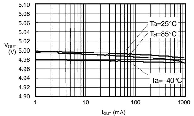
3. Temperature (Ta) - Output Voltage (V<sub>OUT</sub>) Characteristics
