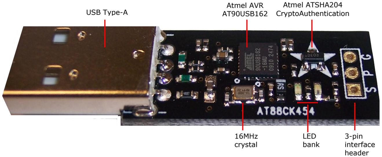
Figure 1-2. Bottom side components placement
