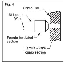
Crimp the ferrule by closing the handles until the controlled cycle mechanism releases. Upon release, the handles will open automatically and the crimped ferrule can be removed.
