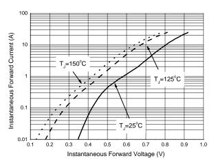
Figure 1. Typical Forward Voltage Per Diode
