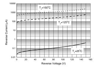
Figure 2. Typical Reverse Current Per Diode
