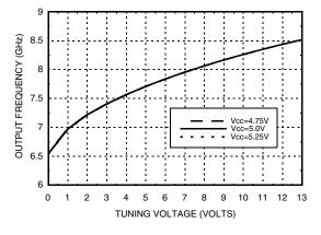
Sensitivity vs. Tuning Voltage, Vcc= +5V
