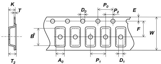
Fig.6 Emboss Carrier Tape Dimensions
