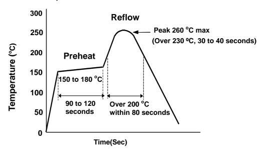
Fig.5 Recommended IR Reflow profile
