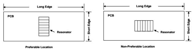
**Fig.10 Mounting Direction**
