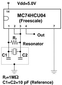
Fig 1 Standard Measuring Circuit
