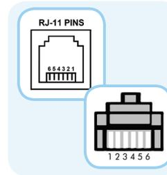
If using RJ11 cable, straight or crossover cable are both supported. (Only pins 3 and 4 are actually used.)
