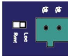
The DIP switch is on top of the device.
