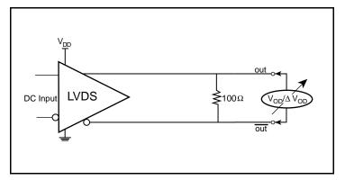
**Differential Output Voltage Setup**
