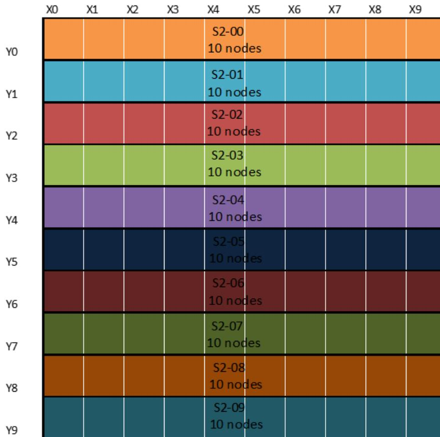
The Lumped Sensors arrangement for row and column sensors are formed by grouping the individual sensors on each row as one set of lumped sensors and similarly for the nodes on each column are grouped as another set of lumped sensors. Optimized bursting algorithm identifies rows/columns that needs to be burst from the previous stage and are burst accordingly.
