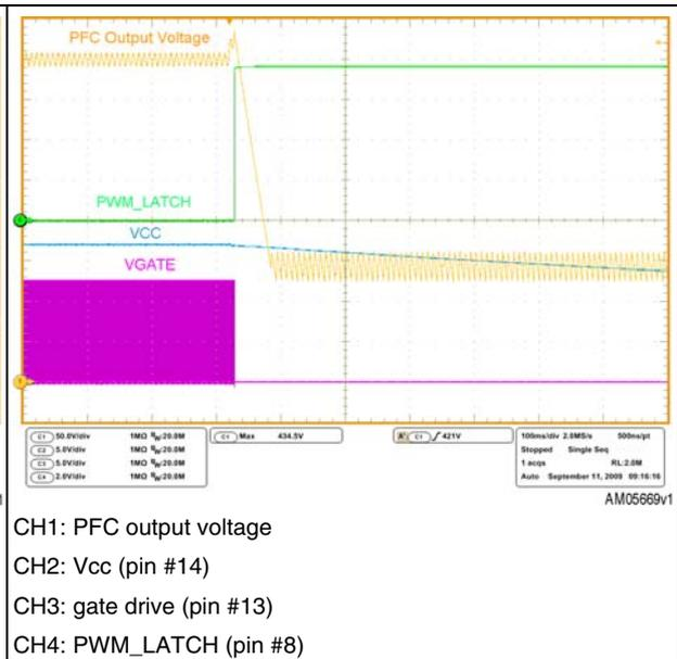
The event of an open loop is captured in [Figure 30](#). We can notice the protection intervention, latching the operation of the L6563S. As mentioned previously, to restart the system the input power must be recycled.
