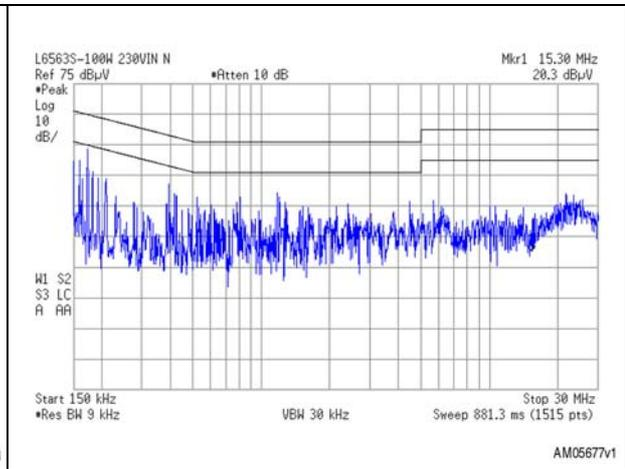
As visible in the diagrams, in all test conditions there is a good margin of the measures with respect to the limits. The measurements have been done in peak detection to speed up the sweep, otherwise taking a long time. Please note that the measurements done in quasi-peak or average as required by the regulation will be much lower because of the jittering effect of the TM control that cannot be evaluated in peak detection.
