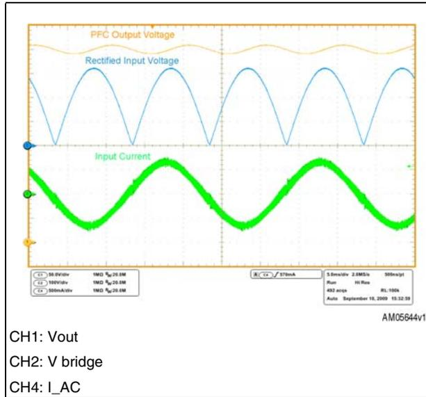
**Figure 6. EVL6563S-100W TM PFC: input current waveform at 100 V, 50 Hz, 100 W load**
