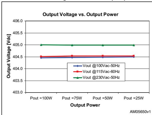
The measured output voltage at different line and static load conditions is shown in [Figure 11](#). As visible, the voltage is very stable over the entire input voltage and output load range.
