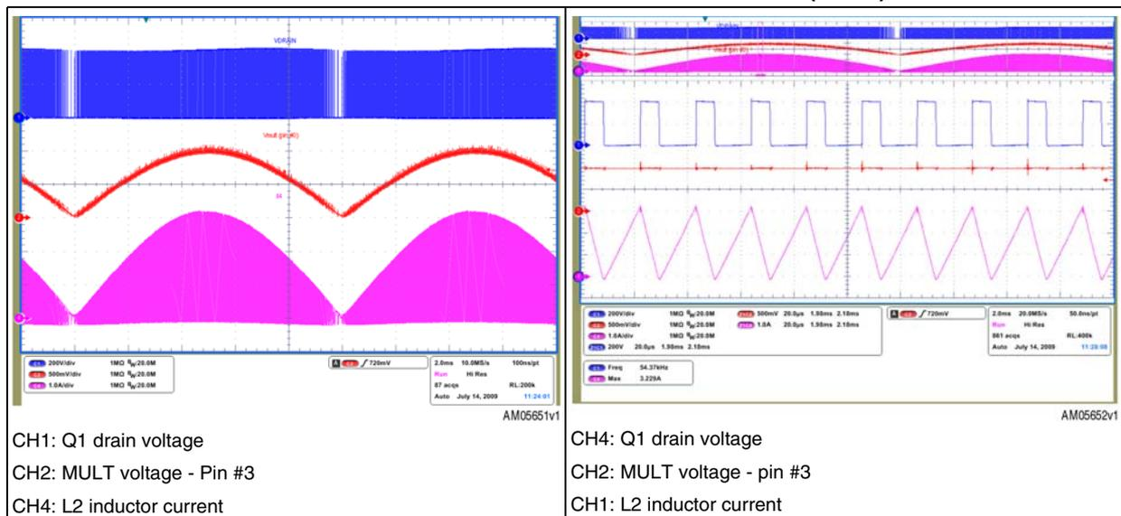
In [Figure 13](#) and [15](#) the detail of the waveforms at switching frequency allows measuring the operating frequency and the current peak at top of the input sine wave during operation at 100 Vac and 230 Vac. The multiplier waveform has been captured as a reference.
