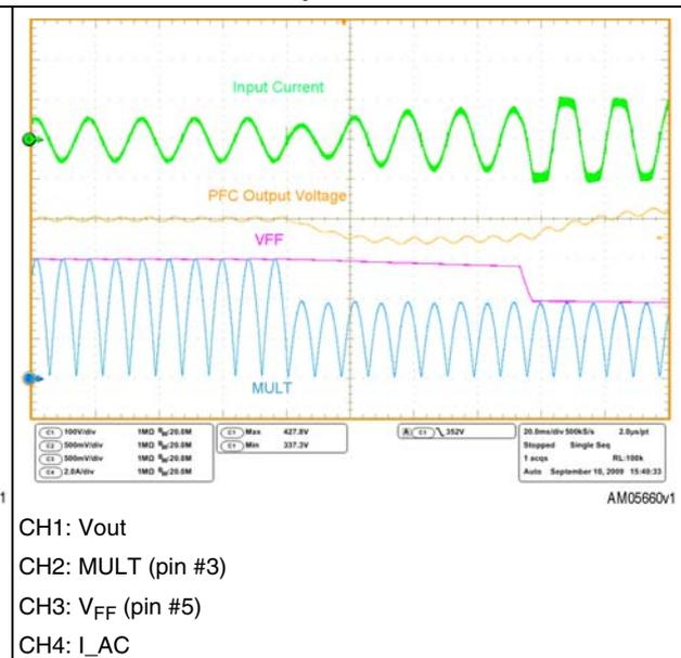
Comparing [Figure 22](#) and [23](#) we can see that the input current of the latter has a better shape and the 3<sup>rd</sup> harmonic current distortion is not noticeable. This demonstrates the benefits of the new voltage feed-forward circuit integrated in the L6563S. Allowing a fast response to mains disturbances but using a quite long  $V_{FF}$  time constant provides also very low THD and high PF at same time as confirmed by the measurements below.
