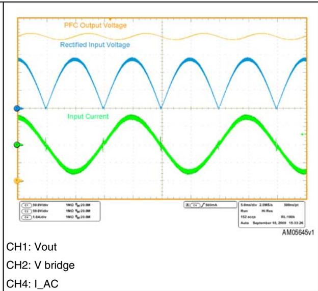
The power factor (PF) and the total harmonic distortion (THD) have been measured too and the results are shown in [Figure 7](#) and [8](#). As visible, the PF remains close to unity throughout the input voltage mains and the total harmonic distortion is very low.
