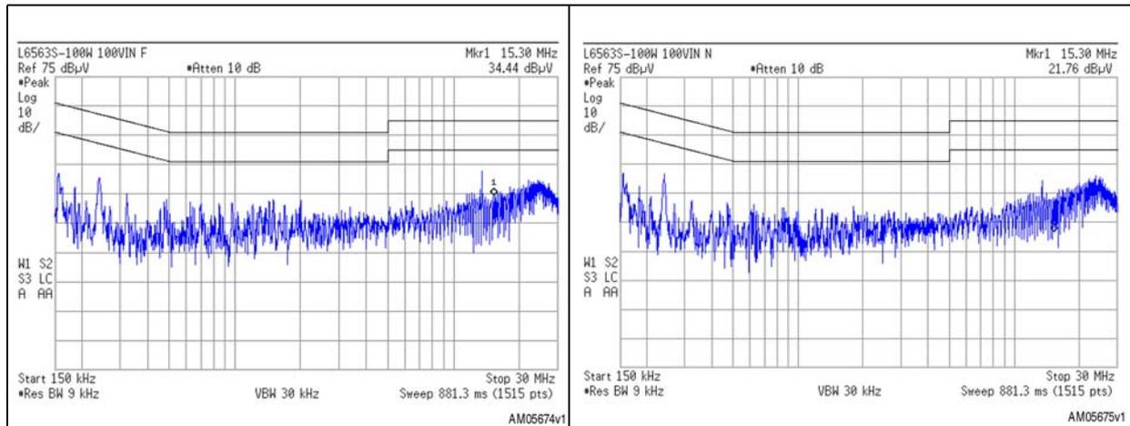
**Figure 37. EVL6563S-100W TM PFC CE peak measurement at 230 Vac, 50 Hz, full load, phase**
