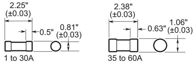
**Description:** Advanced protection Class J current-limiting, fast-acting fuses.
