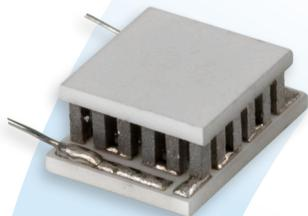
The OptoTEC™ Series is a miniature thermoelectric module (TEM). This product series is primarily used in applications to stabilize the temperature of sensitive optical components in telecom and photonics industries.
