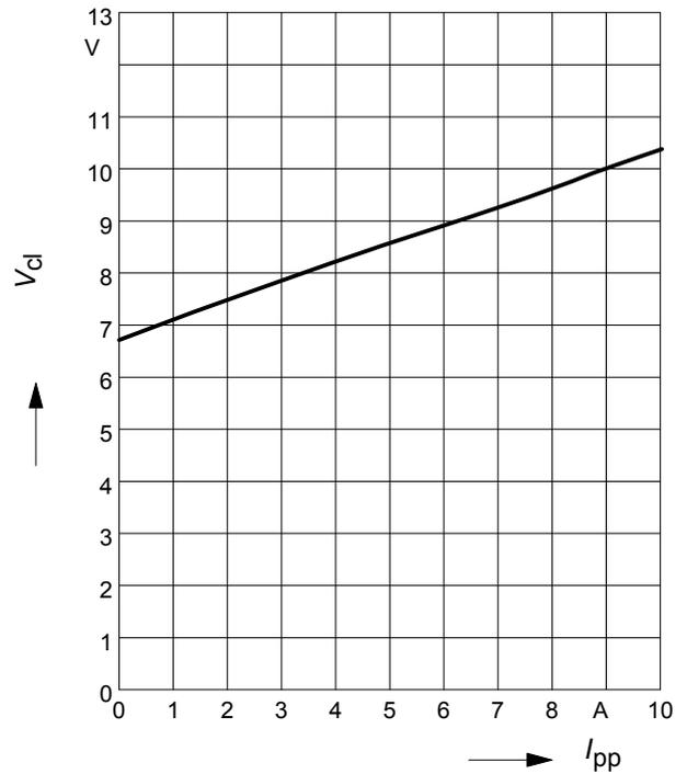
**Forward clamping voltage  $V_{FC} = f(I_{pp})$**
