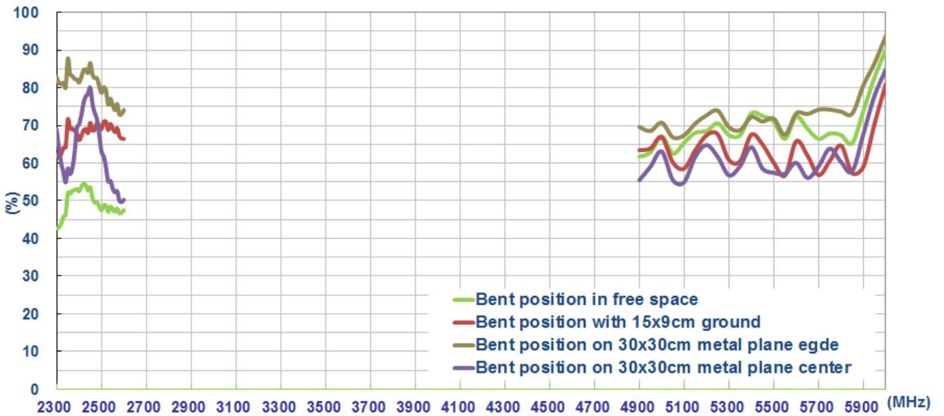
**Figure5.** Efficiency of GW.05 antenna with bent position
