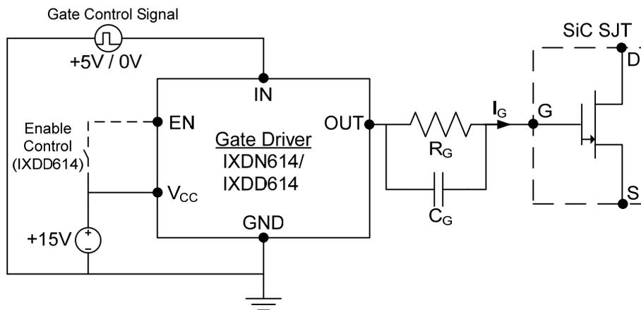
**Figure 14: Recommended Gate Driver Configuration (Option #2)**
