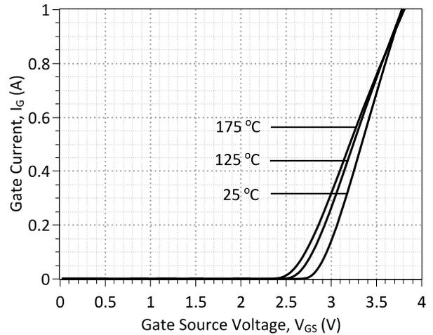
Figure 4: Typical Gate Source I-V Characteristics vs. Temperature
