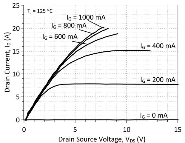
**Figure 2: Typical Output Characteristics at  $125\text{ }^\circ\text{C}$**
