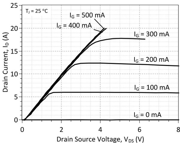
**Figure 1: Typical Output Characteristics at  $25\text{ }^\circ\text{C}$**
