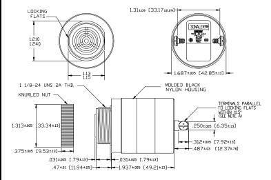
NOTE A: TERMINALS-032 BRASS TIN PLATED, TAPPED FOR #6-32 SCREW, TWO #6-32 NICKLE PLATED BRASS SCREWS INCLUDED, WILL ACCEPT 1/4' QUICK CONNECT.
