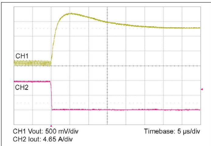
Figure 11 — 9.4 – 0 A load step with 100  $\mu\text{F}$  input capacitor and no output capacitor.
