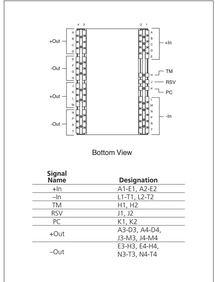
Figure 14 — BCM™ bus converter pin configuration
