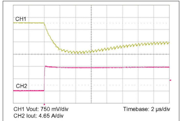
Figure 10 — 0 – 9.4 A load step with 100  $\mu\text{F}$  input capacitor and no output capacitor.
