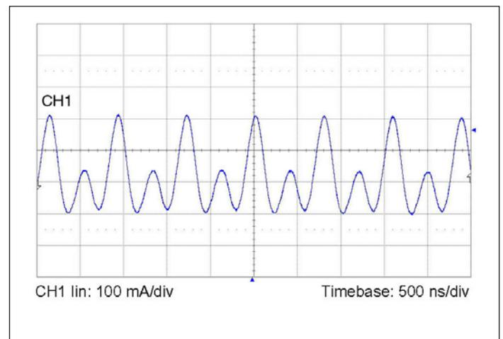
**Figure 4** — Input reflected ripple current at full load and 48 V<sub>IN</sub>
