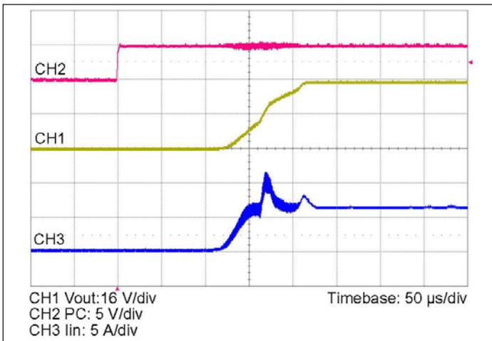
**Figure 1** — Inrush transient current at full load and 48 V<sub>IN</sub> with PC enabled
