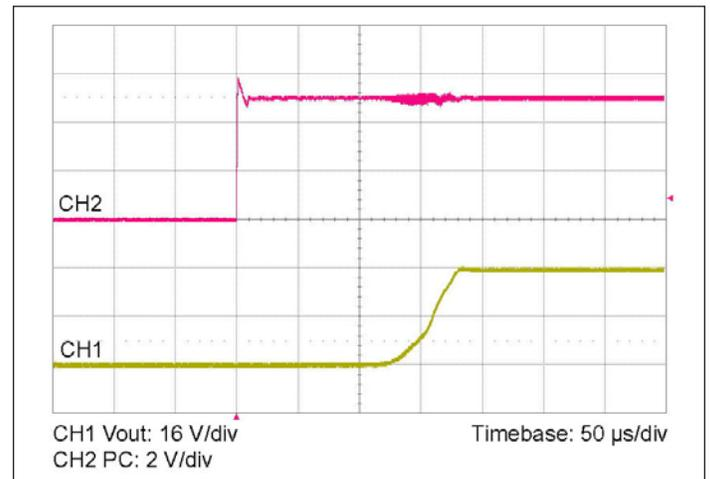
**Figure 2** — Output voltage turn on waveform with PC enabled at full load and 48 V<sub>IN</sub>
