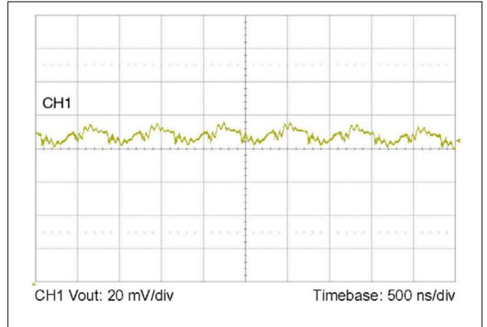
Figure 8 — Output voltage ripple at full load and 48  $V_{IN}$  with 4.7  $\mu\text{F}$  ceramic external bypass capacitor and 20 nH of distribution inductance.
