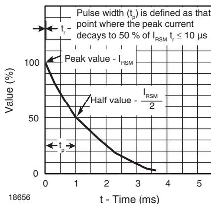
Fig. 2 - Pulse Waveform
