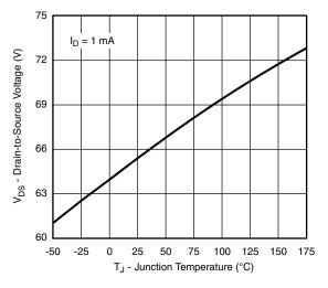
Drain Source Breakdown vs. Junction Temperature
