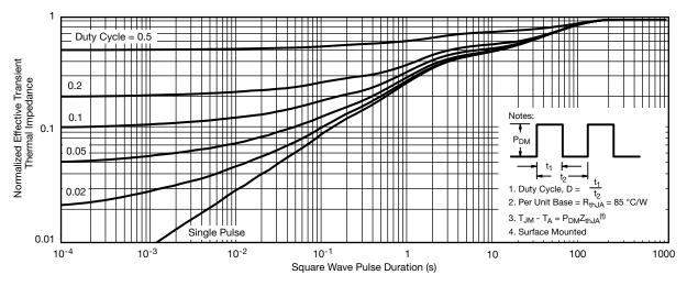
Normalized Thermal Transient Impedance, Junction-to-Ambient
