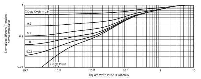
Normalized Thermal Transient Impedance, Junction-to-Foot
