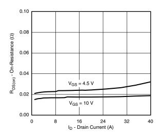
On-Resistance vs. Drain Current
