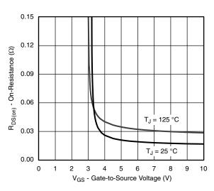
On-Resistance vs. Gate-to-Source Voltage
