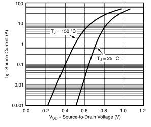
Source Drain Diode Forward Voltage
