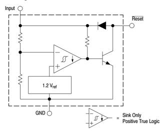
This device contains 21 active transistors. Figure 1. Representative Block Diagram
