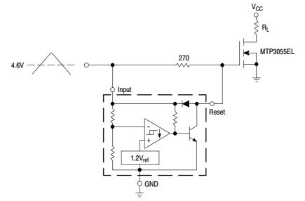
Overheating of the logic level power MOSFET due to insufficient gate voltage can be prevented with the above circuit. When the input signal is below the 4.6 V threshold of the MC34064, its output grounds the gate of the  $L^2$  MOSFET.
