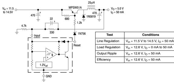
Figure 13. Low Power Switching Regulator
