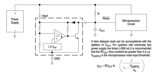
Figure 9. Low Voltage Microprocessor Reset
