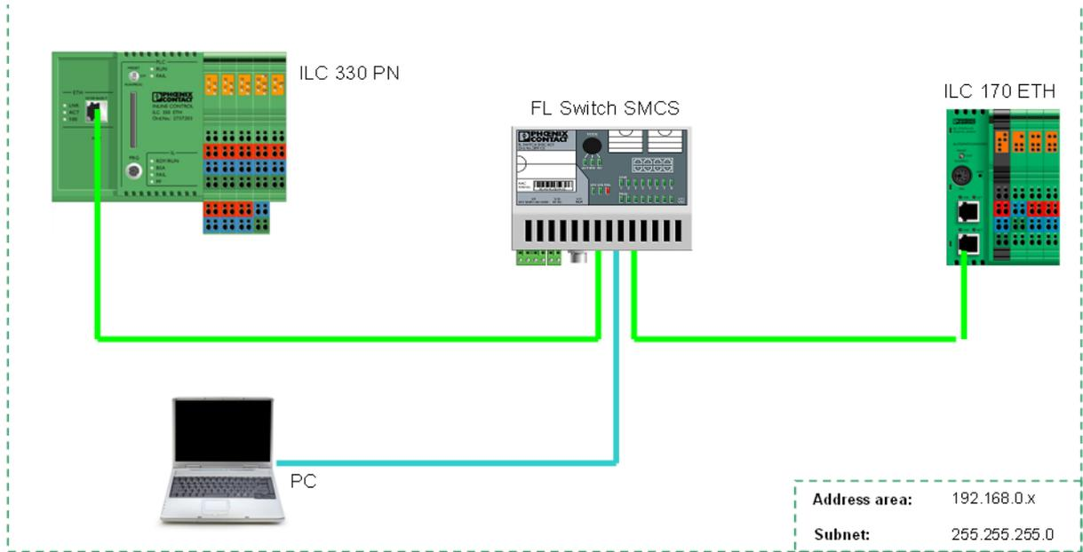
Figure 3-4 Typical application, all devices in one network
