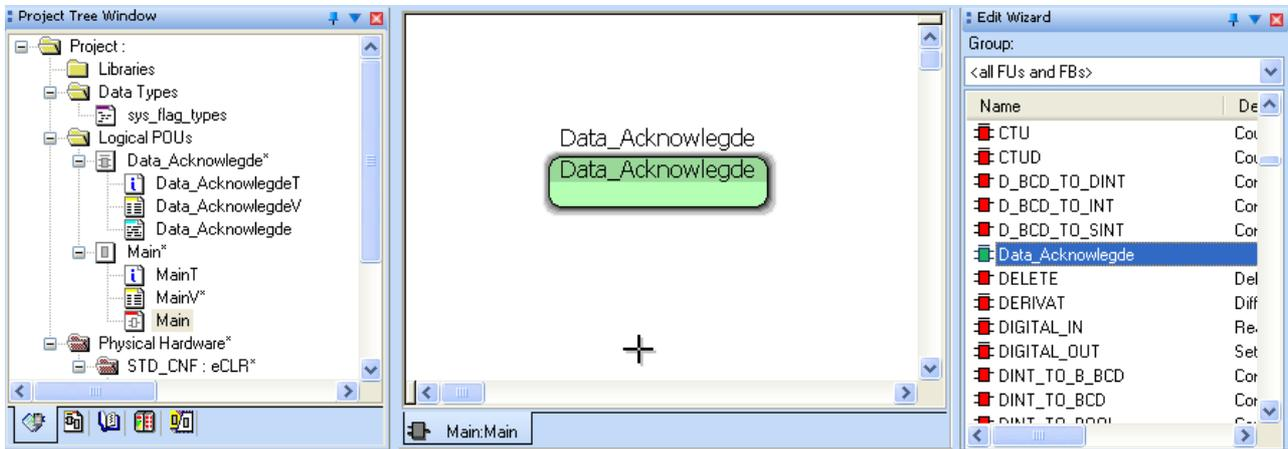
Figure 3-13 Inserting the function block into the worksheet
