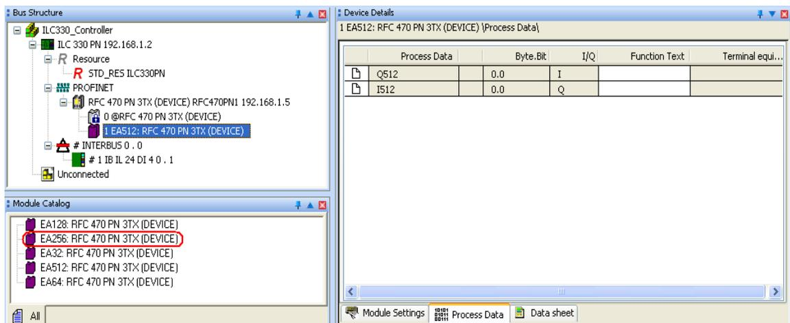
Figure 4-26 Process data of the PROFINET IO device
