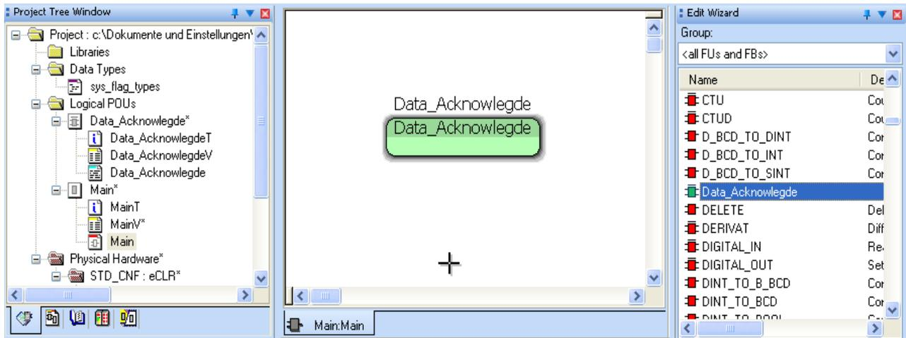
Figure 4-10 Inserting the function block into the worksheet
