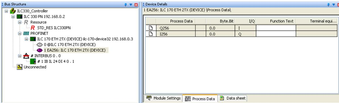
Figure 3-19 Process data of the PROFINET device
