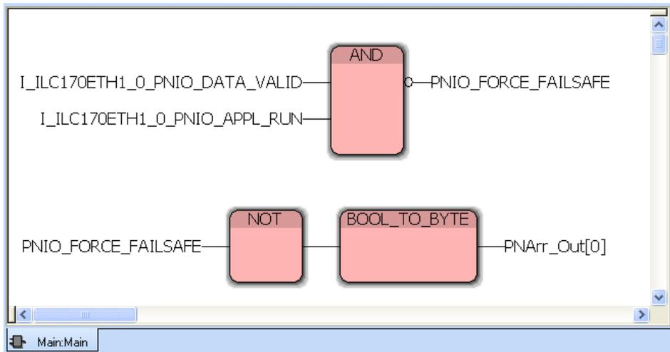
Figure 4-31 Inserting and linking variables
