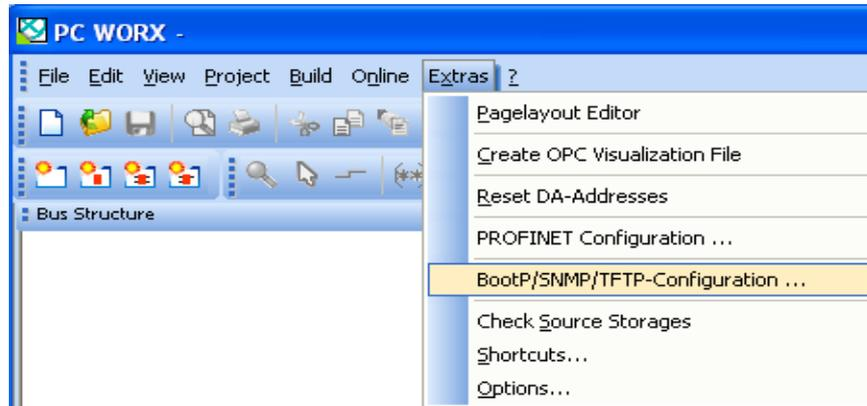
Figure 4-34 Selecting "Extras/BootP/SNMP/TFTP-Configuration..."
