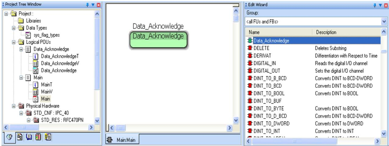
Figure 4-19 Inserting the function block into the worksheet
