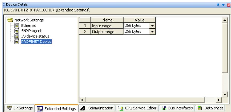
Figure 3-38 Input/output data ranges
