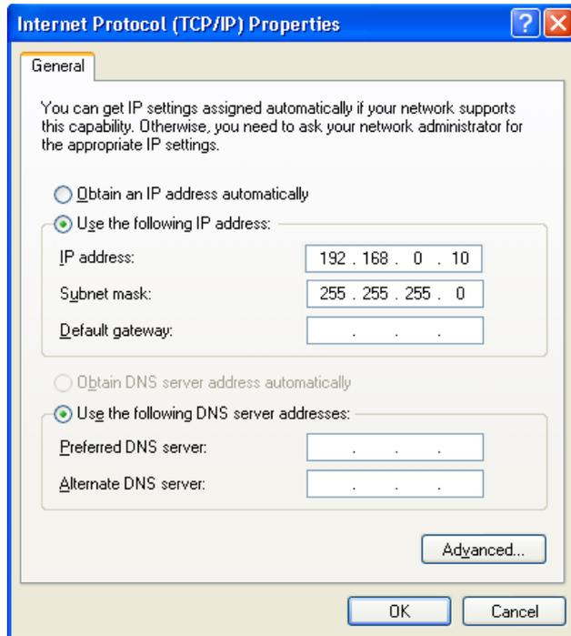
Figure 3-25 Assigning an IP address
