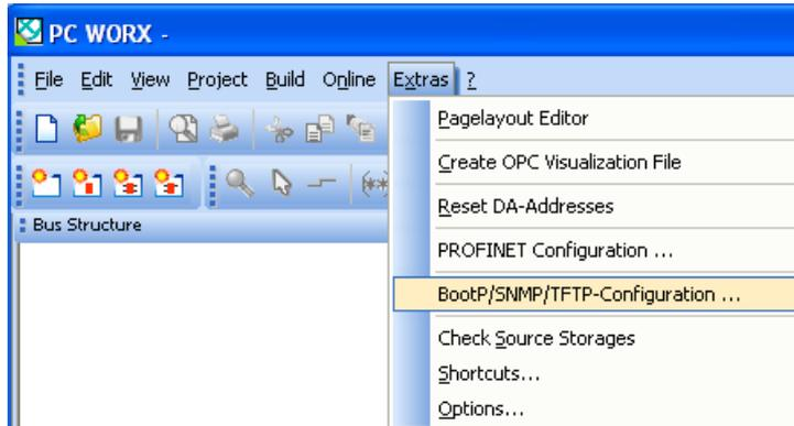
Figure 3-27 Selecting "Extras/BootP/SNMP/TFTP-Configuration..."
