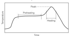
For soldering (Example : Sn/Pb)
