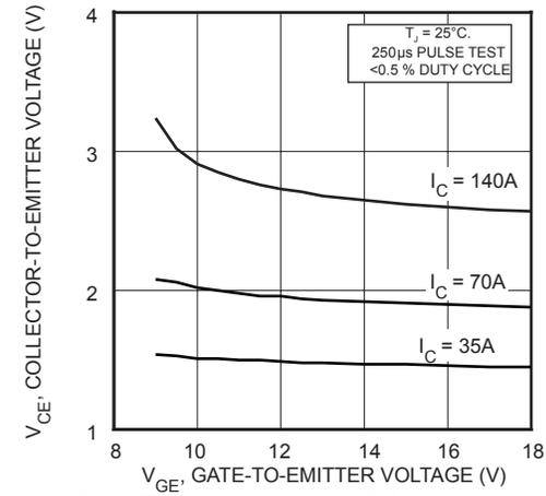
FIGURE 7, On State Voltage vs Gate-to-Emitter Voltage
