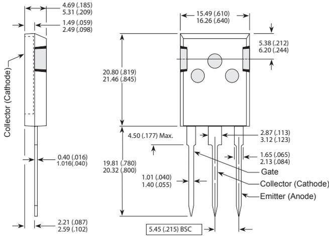
These dimensions are equal to the TO-247 without the mounting hole.
