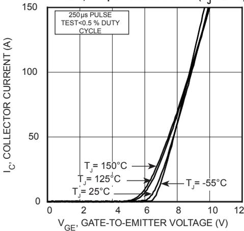
FIGURE 6, Transfer Characteristics
