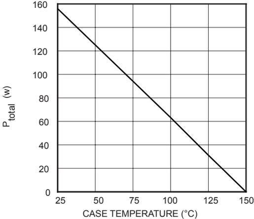
Figure 21. Maximum Power Dissipation vs. Case Temperature
