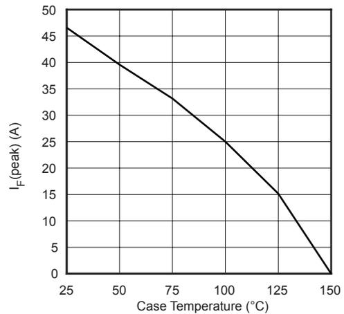
FIGURE 20. Maximum Forward Current vs. Case Temperature
