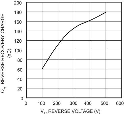
Figure 22. Reverse Recovery Charge vs. V<sub>R</sub>
