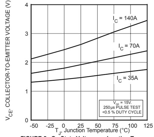
FIGURE 5, On State Voltage vs Junction Temperature
