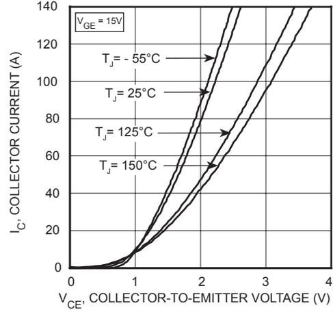
FIGURE 3, Saturation Voltage Characteristics ( $T_J = 25^{\circ}C$ )
