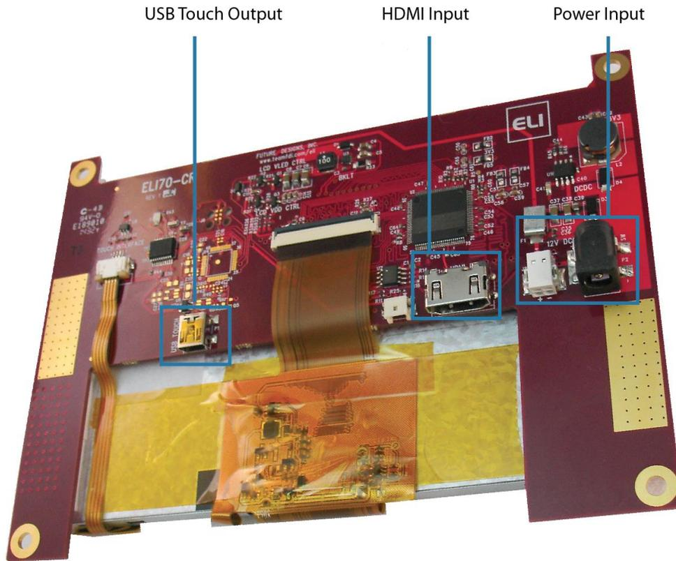
*Power may be supplied either via the 2-pin terminal block J8 or via the 2.1mm power jack P2 (center positive)*
